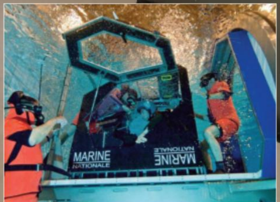
An SSL METS being used to train pilots of the French Marine Nationale in underwater escape techniques. METS are used to train fast jet and helicopter pilots.
